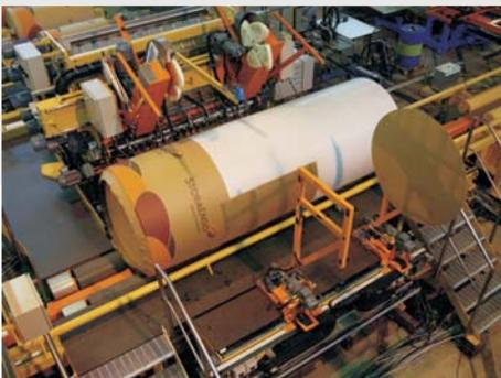
Jumbo size Rolls are wrapped with the Optima Method.
